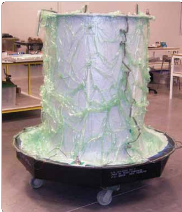
Figure 7-36. Bagging of complex part.
