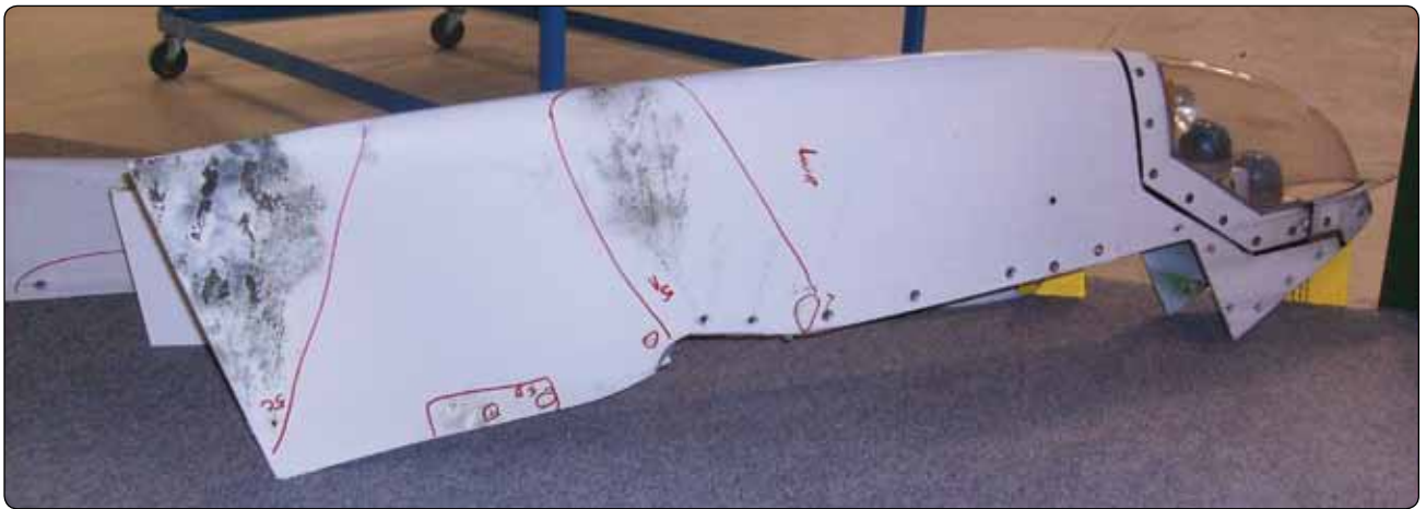
Figure 7-22. Erosion damage to wingtip.
