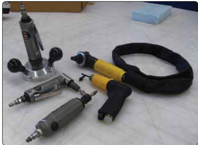
Figure 7-32. Air tools used for composite repair.
