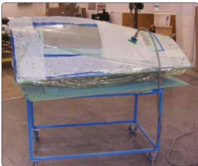
Figure 7-52. Envelope bagging of repair.
