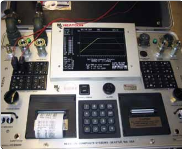
Figure 7-40. Heat bonder equipment.
