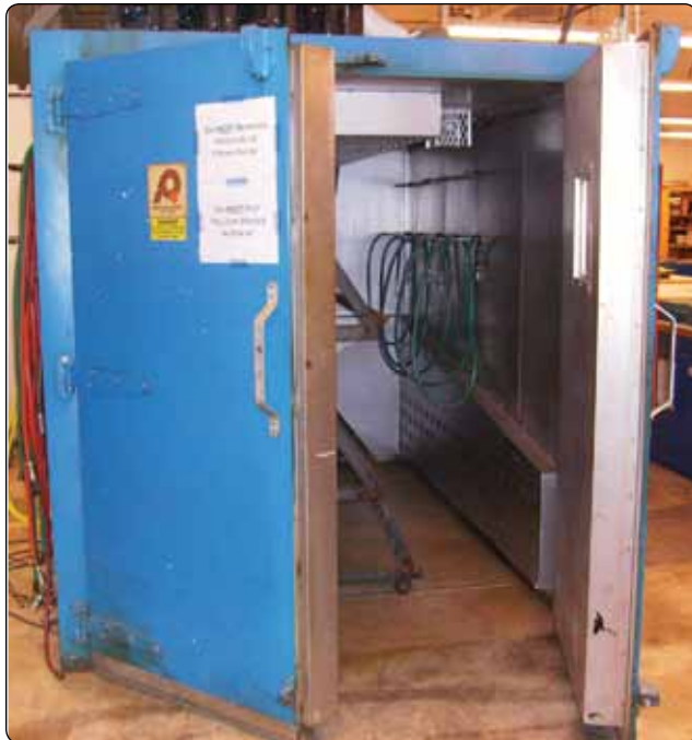
Figure 7-38. Walk-in curing oven.
