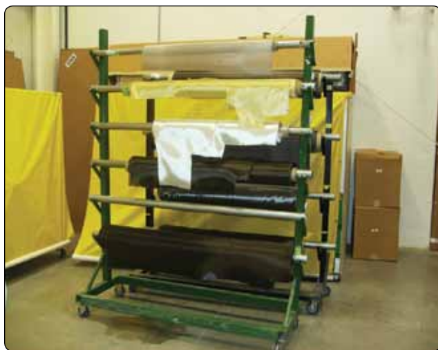
Figure 7-12. Dry fabric materials (top to bottom: aluminum lightning protection mesh, Kevlar®, fiberglass, and carbon fiber).
